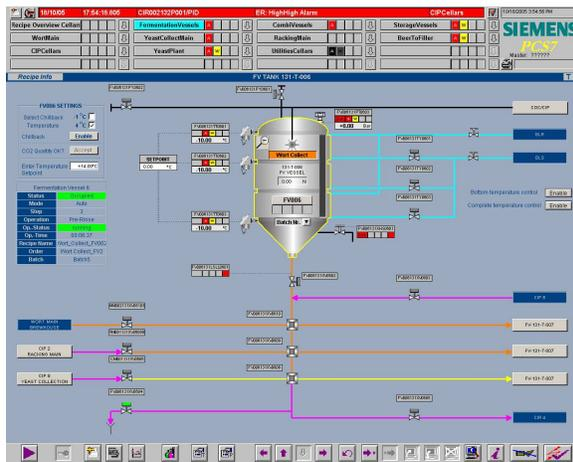
Figure 5 – One of the Vessels with associated devices as displayed on the SCADA.
